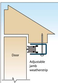
**Figure 2.** Example of adjustable weatherstripping (FEMA 577).
